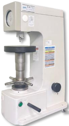
Hardness meter (Rockwell type)
