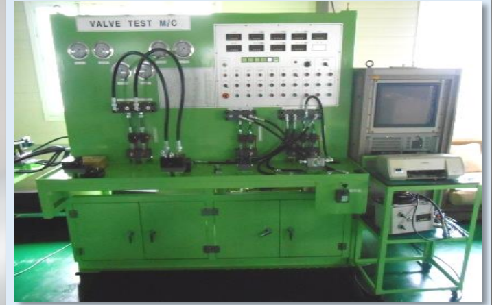
Double Pilot Check V/V Test Bench
