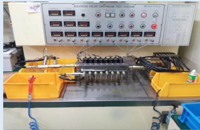
Solenoid V/V Cartridge Test Bench
